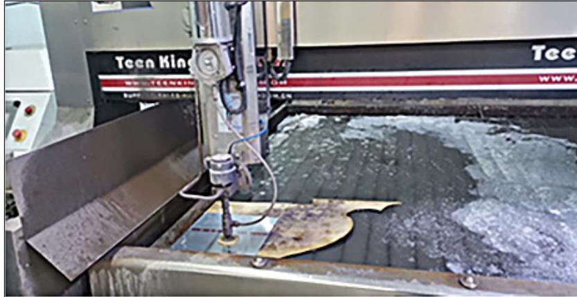
Figure 1. Abrasive water jet machine
